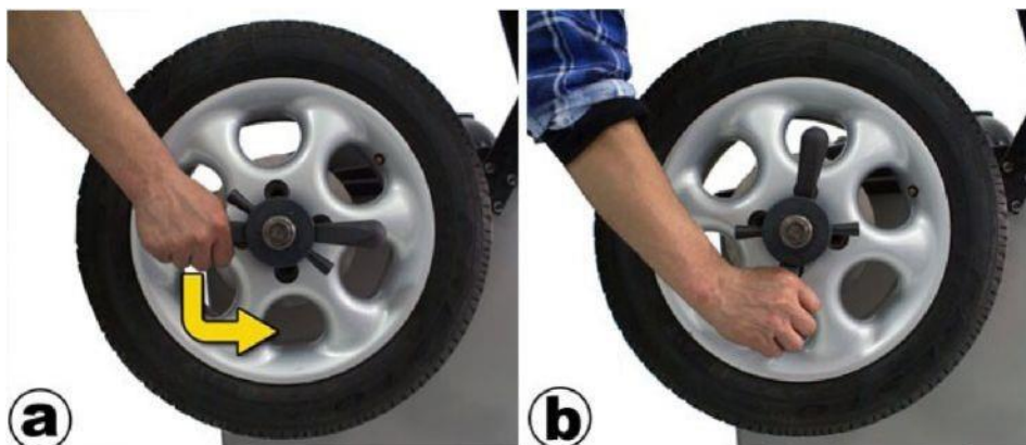
Fig. 9: Removing wheel from the holder.
