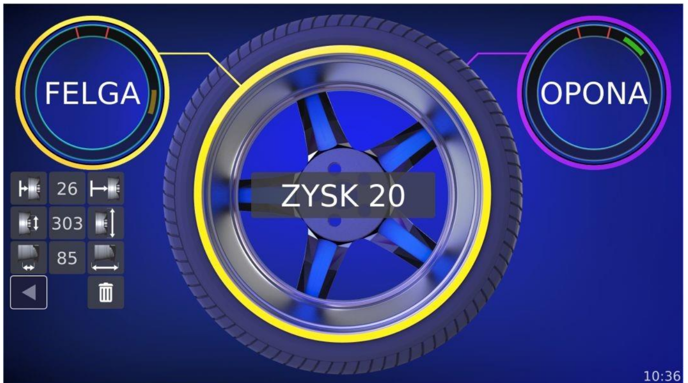
Fig. 26: Sample optimization screen after wheel measurement
