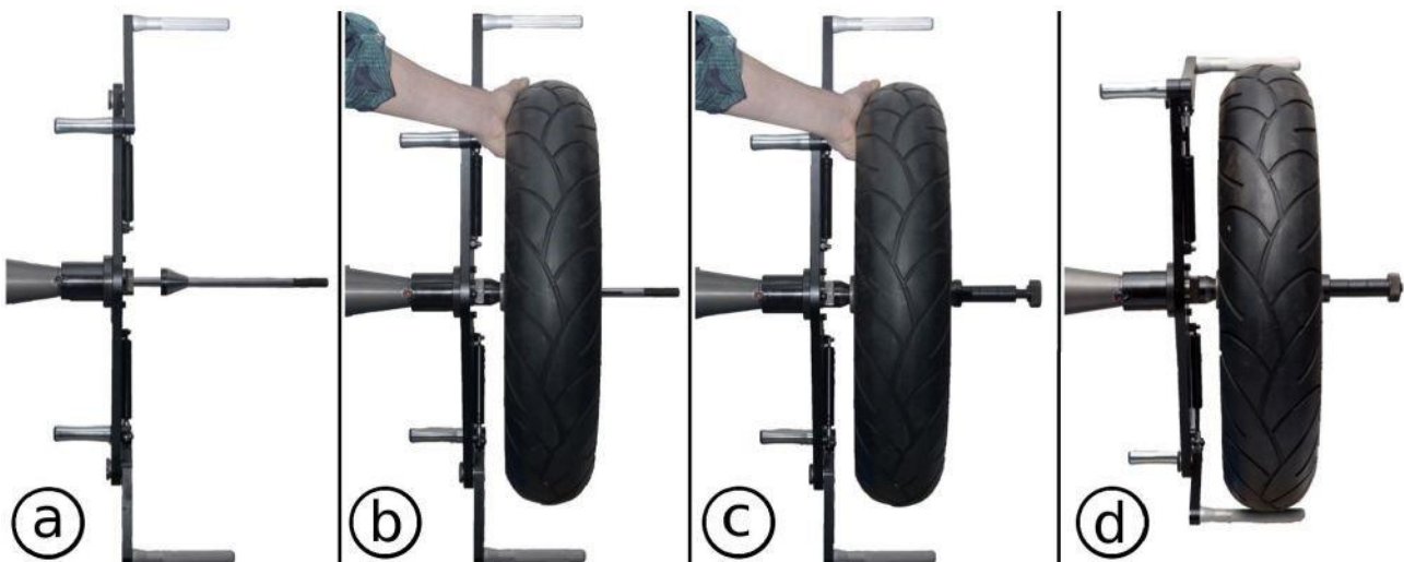
Fig. 14: Motorcycle wheel mounting on the holder.
