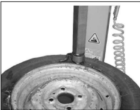
Fig. 8. Head in working position.
