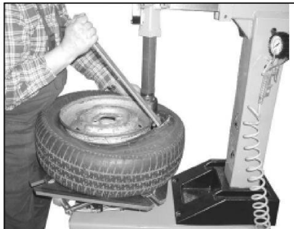
Fig. 9. Pulling bead tyre edge onto bulb.
