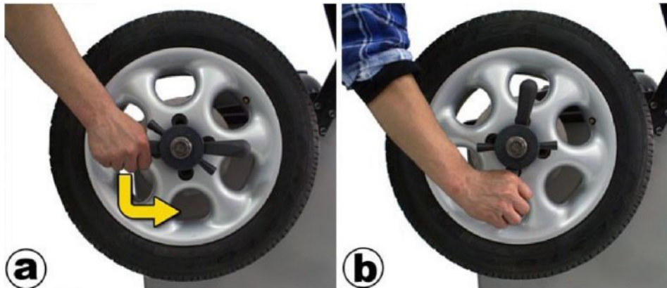
Fig. 9: Removing wheel from the holder.
