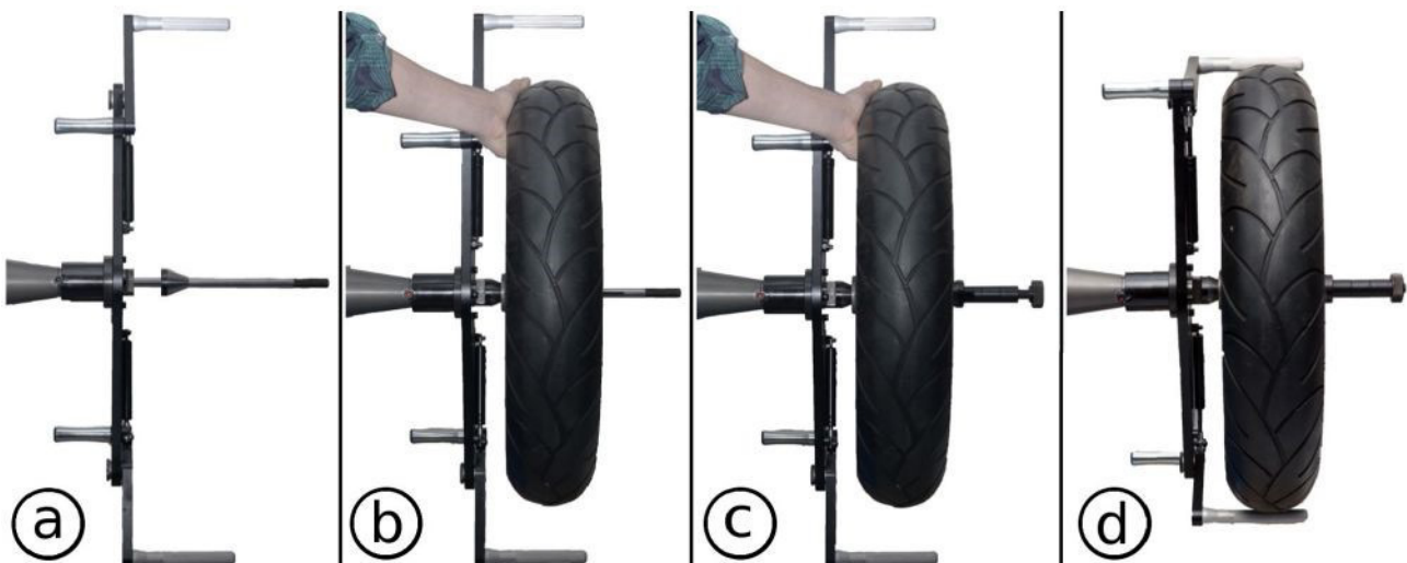
Fig. 14: Motorcycle wheel mounting on the holder.
