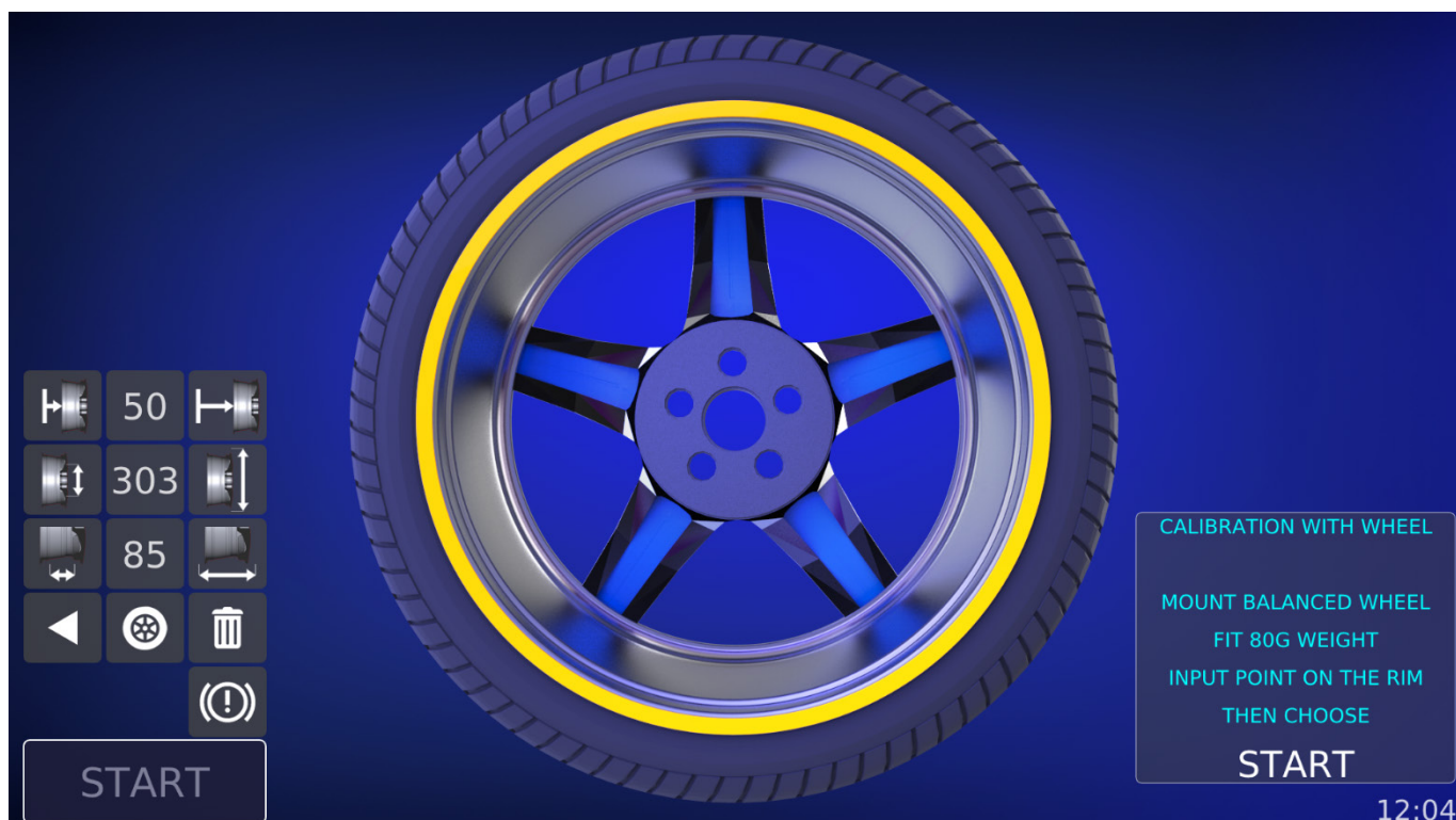
Fig. 28: Calibration with wheel
