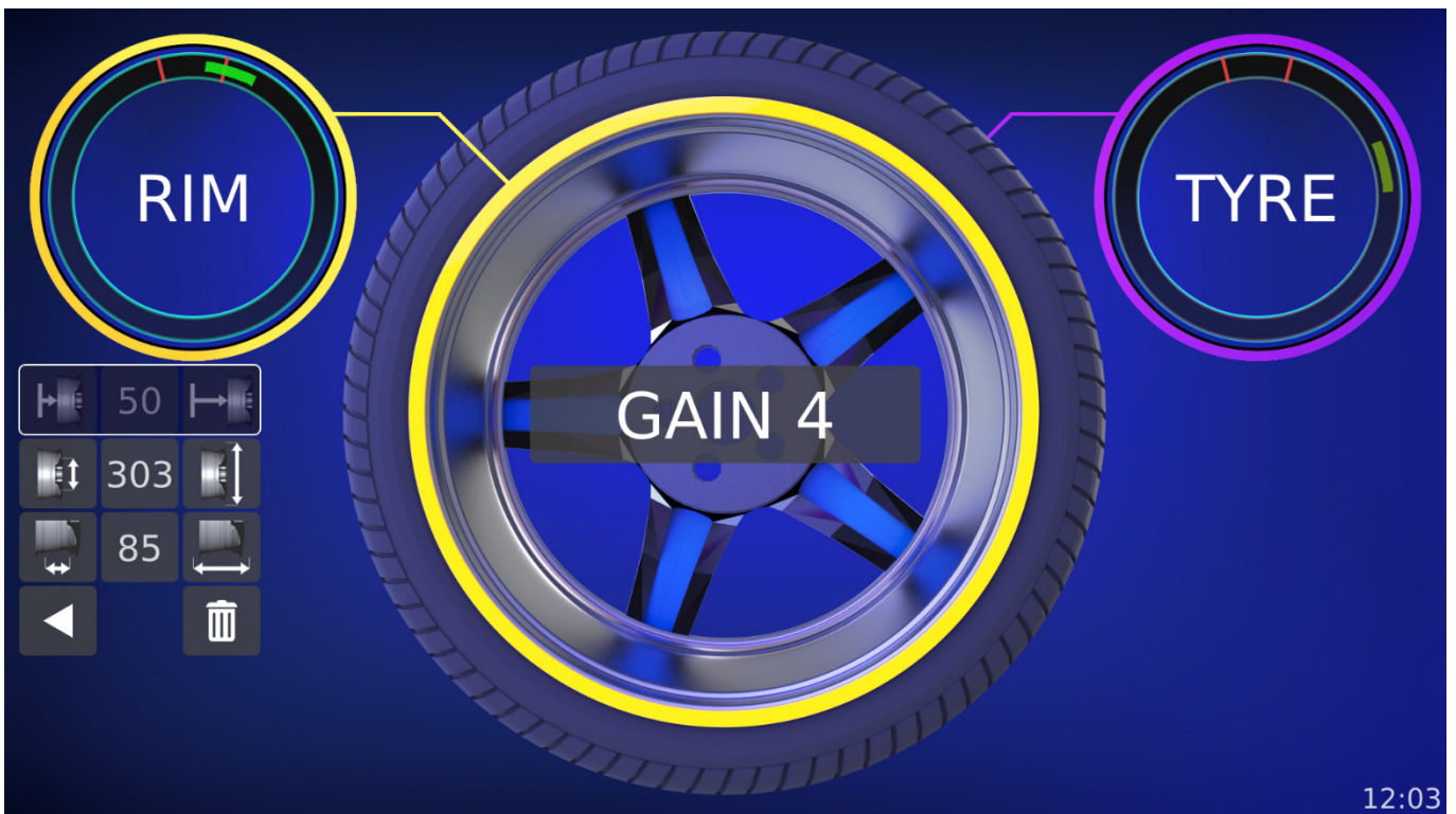
Fig. 26: Sample optimization screen after wheel measurement
