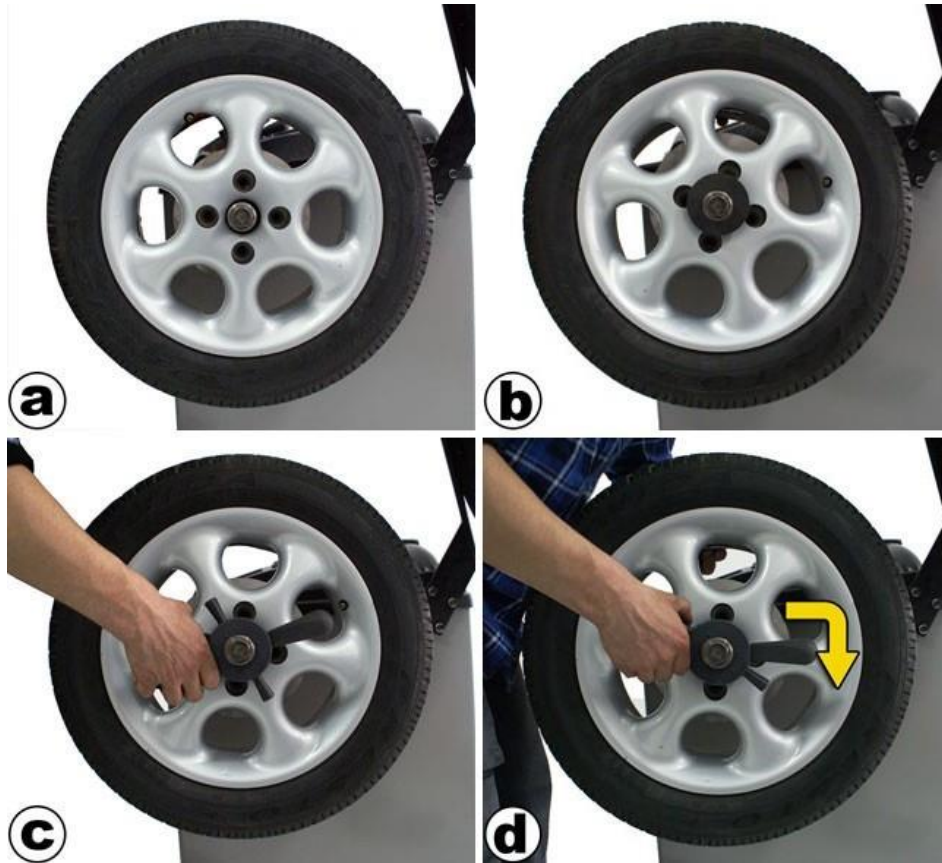
Fig. 5.7 Wheel mounting on balancer's holder
