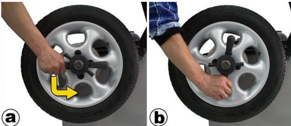
Fig. 5.8 Wheel dismounting from balancer's holder
