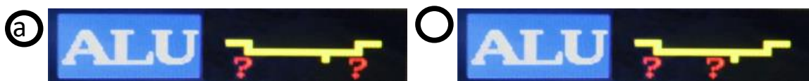
Fig. 7.7 Weight placement icon view a: beginning of second phase b: when continuing adjuster movement into the rim.
