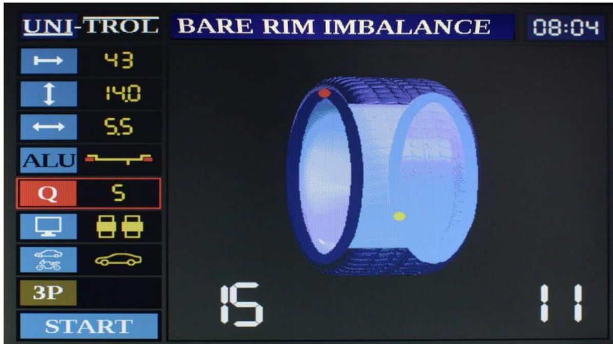
Fig. 6.11 – Optimisation screen – bare rim imbalance.
