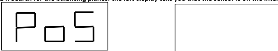
Picture F16.14: Search for the balancing planes: the left display tells you that the sensor is on the internal balancing plane exactly
