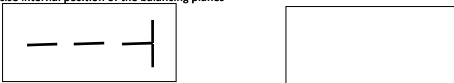
Picture F16.13: Search for the balancing planes: the left display tells you to move the sensor back (move to the left) to find the exact position of the internal balancing plane
